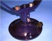
Replace lock wheel with M8 x 10 hexagon screw in the bottom fixing.
