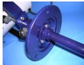
Fasten the under deck mechanism using the 3 off M6 x 16 pan head screws and spring washers.
