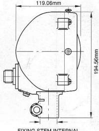
FIXING STEM INTERNAL DIAMETER 28.70mm (1.130")
