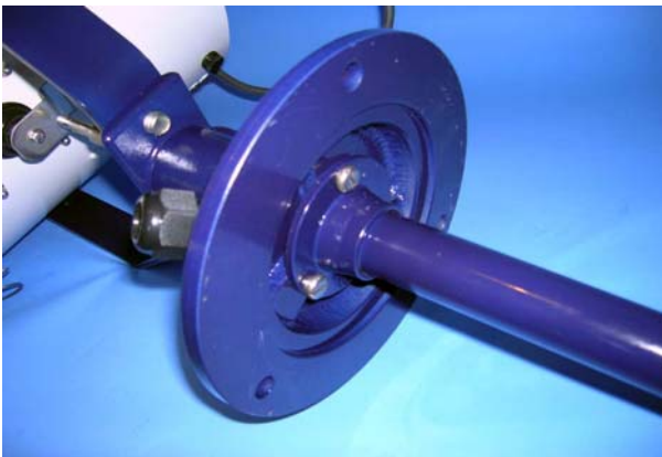
7. Fasten the Under Deck mechanism Using the 3 off M6 X 16 pan head screws and spring washers
