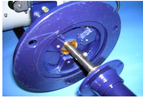
6. Insert the Under Deck through the centre hole making sure it's aligned as photos below
