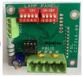
Switching a switch to on, adds the binary value relating to that switch to the address value. With all switches off the value is zero.
