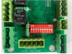
The address value is the sum of the numbers above which are active when the switch is on. For example, if switches 6 and 8 are on, and all others are off, the address value would be 5. Note that switches 1-3 are not used for address selection and should be switched off.
