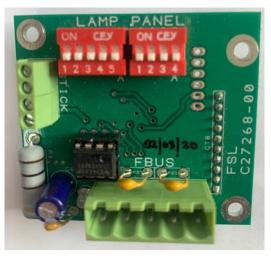
Switching a switch to on, adds the binary value relating to that switch to the address value. With all switches off the value is zero.
