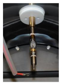
Keep the knurled nut and washer in a safe place as it will be needed later.
