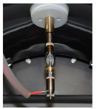
The new lamp must be handled carefully, and a suitable protective cloth must be used when handling the lamp. The front lamp lead can now be re-attached using the M4 knurled nut and washer. Do not overtighten the nut.
