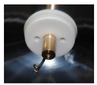
The lamp can now be removed from the rear lampholder by carefully unscrewing it (take care not to lose the M4 spring washer). When fitting the new lamp, the negative end must pass through the ring terminal and M4 spring washer before being screwed back into the lampholder.
