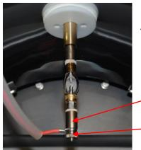
Release the M4 knurled nut and spring washer that secures the front lead to the positive end of the lamp.
