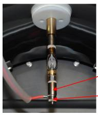
Release the M4 knurled nut that secures the front lead to the positive end of the lamp.
