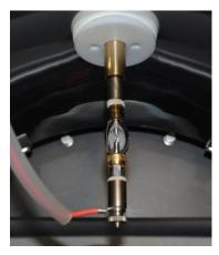
The new lamp must be handled carefully, and a suitable protective cloth must be used when handling the lamp. The front lamp lead can now be re-attached using the M4 knurled nut. Do not overtighten the nut.
