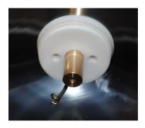
The lamp can now be removed from the rear lampholder by carefully unscrewing it. When fitting the new lamp, the negative end must pass through the ring terminal before being screwed back into the lampholder.
