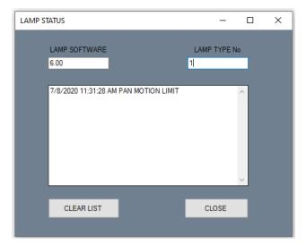
The LAMP STATUS window lists any events or faults relating to the selected lamp. This can be useful for fault diagnosis. The list can be cleared allowing all events after a given time to be reported. The LAMP STATUS window also displays the currently selected lamps software version and lamp type No
