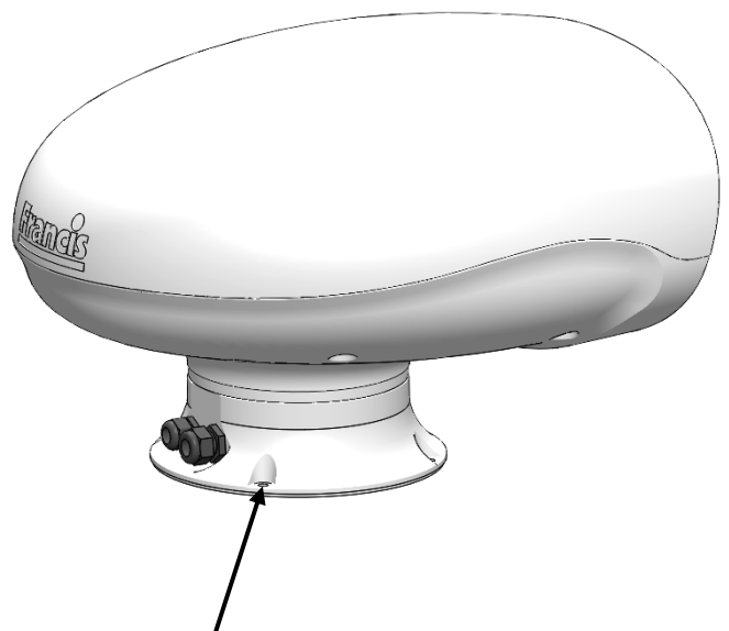
Base Fixings, 4 Holes Ø8.2 Equally Spaced on a Ø220.00
