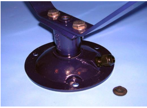
5. Remove the Blanking Plug from the Bellows Bottom Bush.
