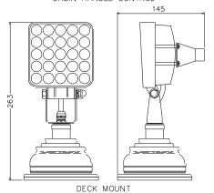
Base fixing details: 3 holes Ø6.4 on a 108 P.C.D. Under deck control clearance hole Ø45. HV transformer 230x 140 x 99mm
