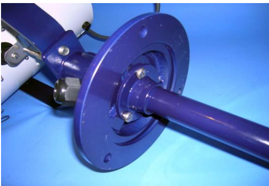
7. Fasten the Under Deck mechanism Using the 3 off M6 x 16 screws and spring washers
